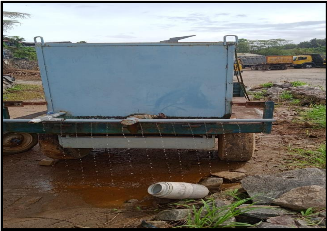
Wetting road using vehicle
